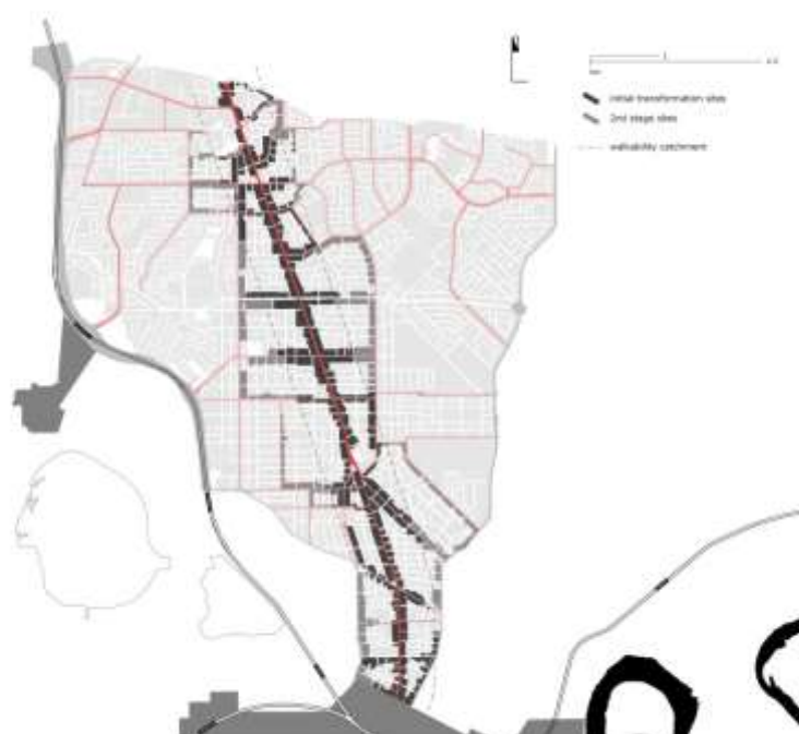
Figure 5: Neighbourhood perimeter development opportunities – only those properties along the busy roadways, where traditional dwelling types perform poorly are selected as possible sites for more intensive development.
