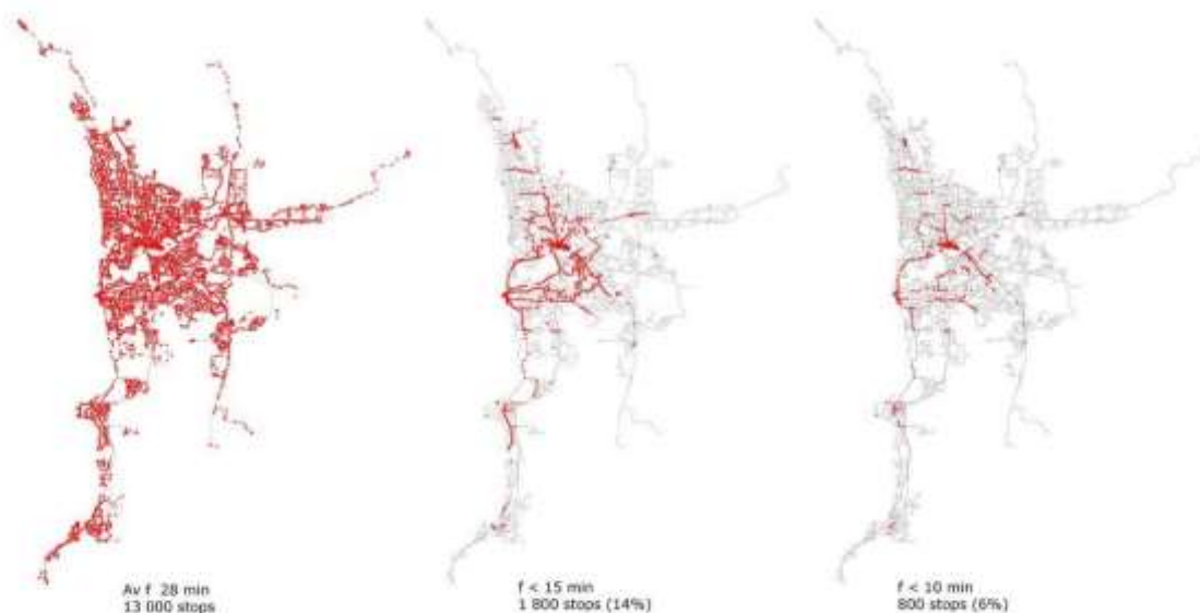
Figure 3 The pattern revealed by increasing the frequency of service of public transport services in Perth (data source – Transperth 2008)
