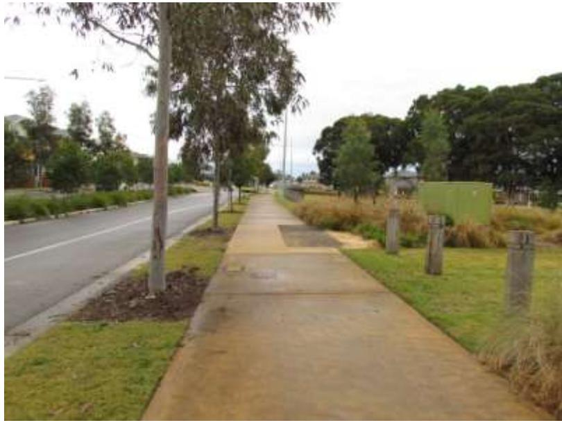
Figure 4 shows a shared pathway located alongside a main road, leading towards the Rouse Hill Town Centre. This shared pathway was assessed as 'good' taking into account material, gradient, connectivity and visibility, though the shading was considered to be poor.
